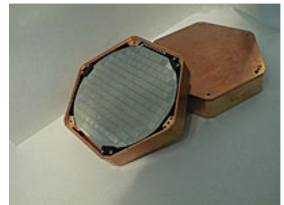
Detectors like this one, from the Cryogenic Dark Matter Search, are placed deep underground to try to detect dark matter.
