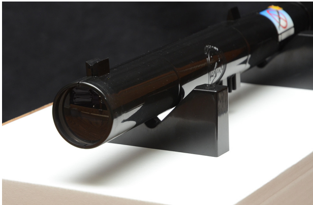
Figure 12: The objective lens in the aperture of a Galileoscope (Image: ASP/Brian Kruse)
