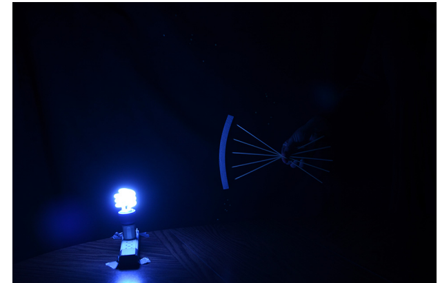
Figure 15c: Bamboo skewers in foam modeling the passage of light rays through a convex lens, resulting in converging light rays (Image: ASP/Brian Kruse)
