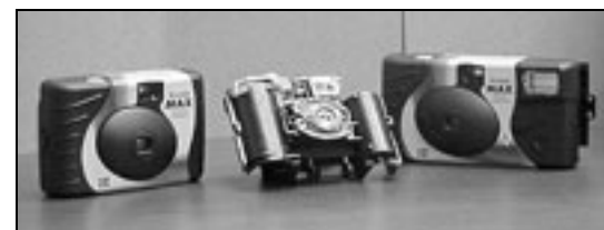
The KODAK One-Time Use cameras with (right) and without (left) the flash unit. The assembly at center is a non-flash unit with its front and back covers removed. Photo courtesy of the authors.
