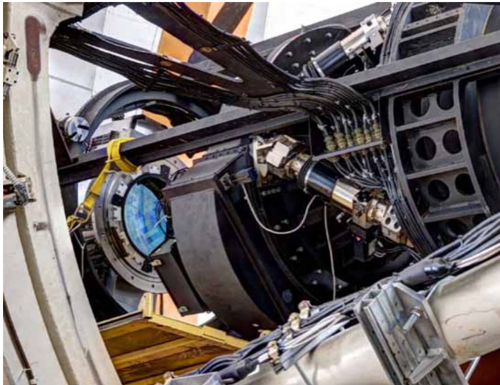
The wide-field DECam camera on the Blanco telescope at Cerro Tololo Inter-American Observatory (CTIO) seen before being inserted into the instrument. Image by T. Abbott & CTIO/NOAO/AURA/NSF.
