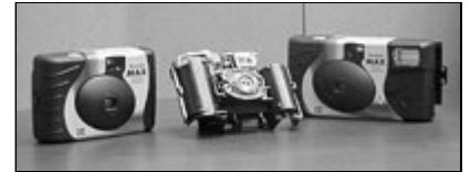
The KODAK One-Time Use cameras with (right) and without (left) the flash unit. The assembly at center is a non-flash unit with its front and back covers removed. Photo courtesy of the authors.
