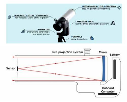
Figure. 2. [top] Five unique features of the eVscope. [bottom] Design of the eVscope.
