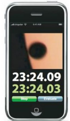
Timing the transit of Venus with the Transit of Venus phone app. Image courtesy of Steven van Roode
