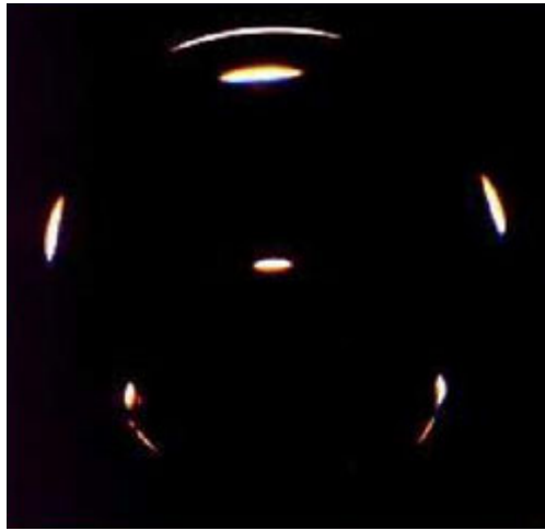
Figure 4. Multiple images of the "quasar" are visible to a camera placed inside the caustic. Photo courtesy of author.
